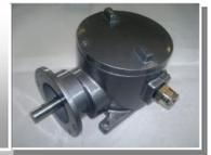
A worm gear and a helical toothed gear combined with one or more pairs of straight toothed gears are used for the transmission of the movement from the input shaft to the internal sensor. Revolution ratios ranging from 1:15 to 1:150 result from the use of different combinations of gear wheels between the input shaft and the output shaft, which is connected to the cams operating the switches.
